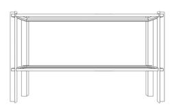
5. Use the wrench and screw the 3rd and  $4^{th}$  table leg to the table top and shelf frames.
